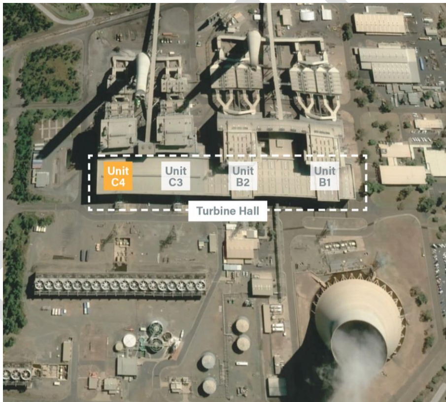
Figure 1 Site layout of Callide B and C power stations showing position of turbine generators 10
