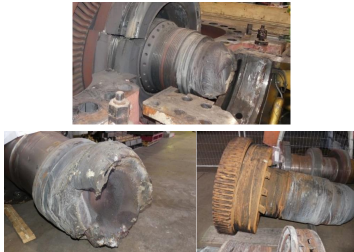
Figure 38 HP turbine, LP turbine and generator shaft damage
